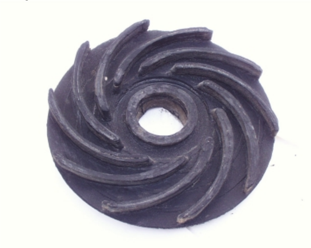
Figure 4 The whole impeller casting mold that is finished manufacturing
