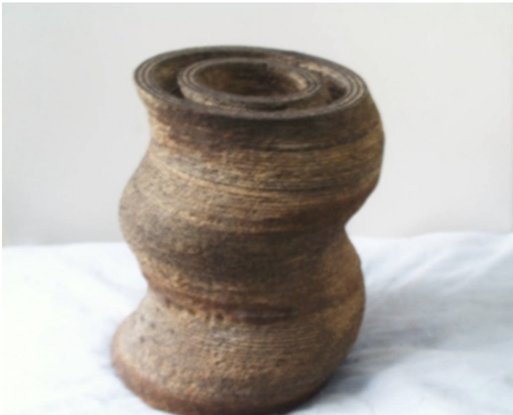
Figure 6 The casting mold of sleeve
