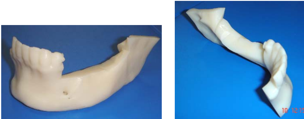
Fig. 2. Mandible bone from Accura 25 (3DSystems SLA machine.)
