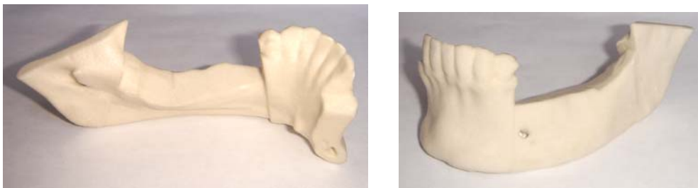
Fig. 6. Mandible bone built by ZCorp 310 machine.
