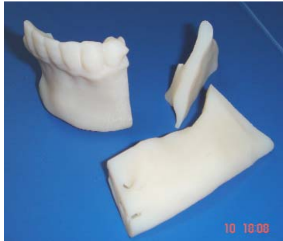
Fig. 5. Mandible bone and graft from FullCure 720 (Eden MJM machine.)
