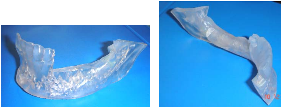
Fig. 3. Mandible bone from Accura 60 (3DSystems SLA machine.)
