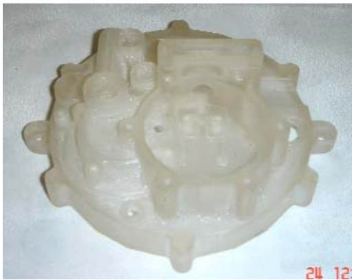
Fig. 4. Rapid prototyping model was developed using Invision 3D printer. This model will be used to re-produce the optimized part with the new dimensions and modified details through the Investment casting techniques.
