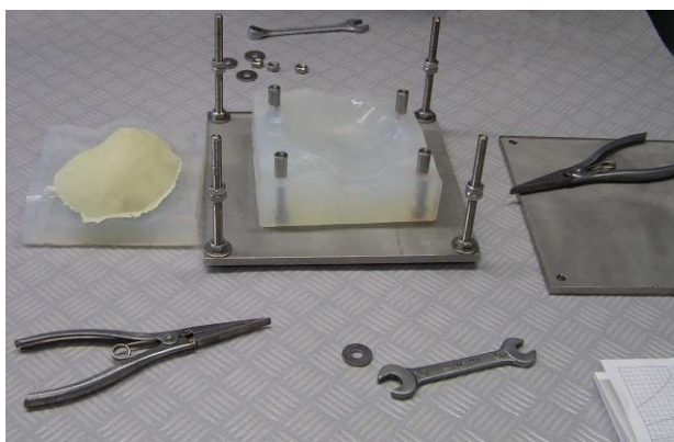
Fig.9. Final mould setup
