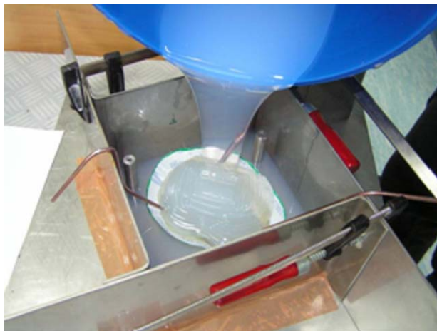
Fig.7. Manufacturing of SRM mould
